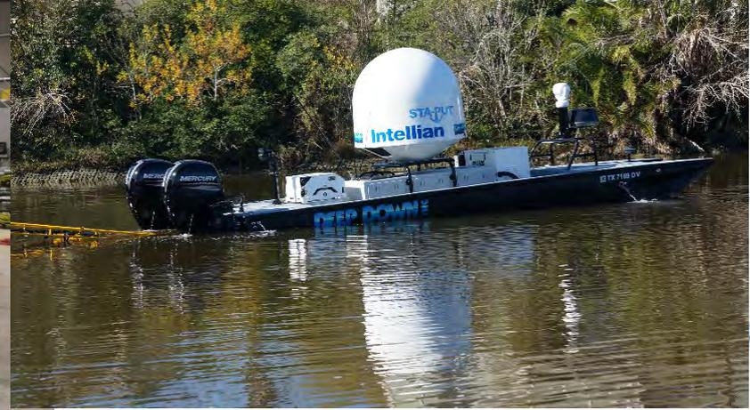
RSV loaded with gyro stabilizer, genset, thrusters, 300hp of Mercruisers, thermal cameras, Intellian world wide satellite, remote via link from anywhere. Plus transmit live video feed
