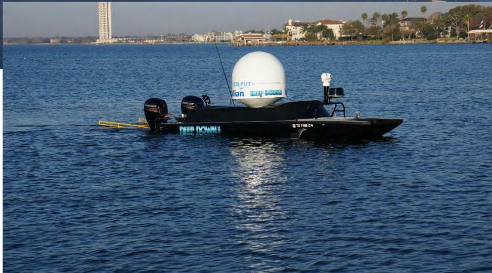
Both the AUV and remote controlled Wahoo support vessel (RSV), complete recent testing in the Galveston Bay area
