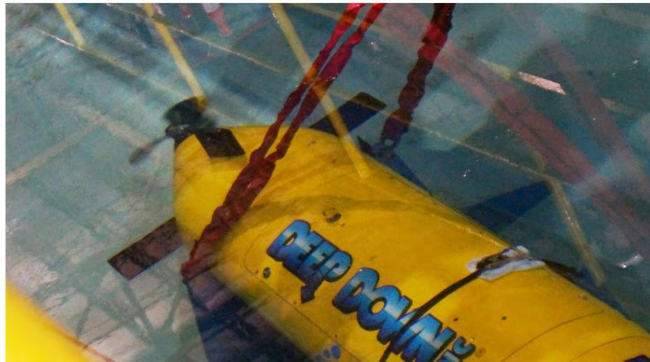
Remote cameras on the test tank and observing the active testing of the DDI AUV with 20% thrust engaged
